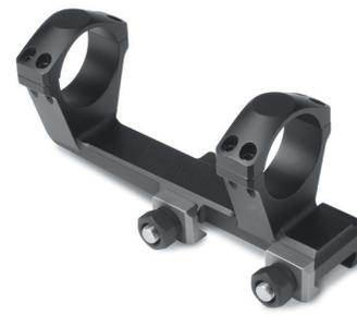
Nightforce X-Treme Duty Unimounts are one-piece scope mounts designed to provide a rock-solid solution that links riflescope to weapon. Manufactured of 7075-T6 aluminum and featuring titanium cross-bolts and clamps, this lightweight but sturdy base is designed to mount to Mil. Std. 1913 rails. Unimounts are compatible with Nightforce Rail Accessory Platform (RAP), Multimount, bubble level and angle degree indicator (ADI) accessories made by Nightforce.
